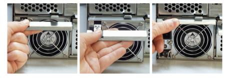
Figure 6. The VTrak M500f/i/p power supply shown above. The M300f/i/p and M200f/i/p are similar
